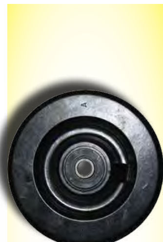
SC-21 10" santoprene on polypropylene wheel. 10"x2.25" .75" plain bearing Load Capacity: 750 lb.
