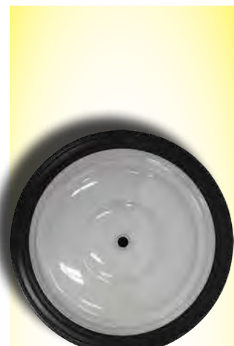
SC-34 12" bolt together, 4-ply pneumatic wheel. 12"x4" .75" ball bearing Load Capacity: 445 lb.
