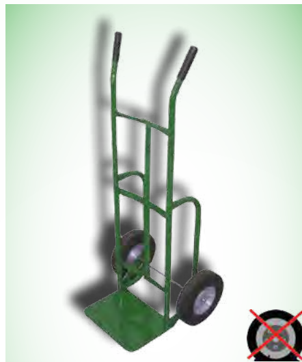
702/702-10 Baseplate: 14"x10" Height: 49" Width: 19"/22" Weight: 39 lb./32 lb. Wheels: SC-8/SC-9A
